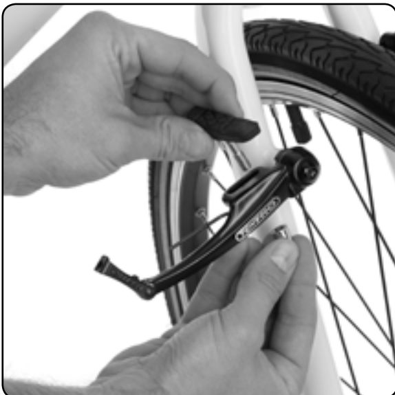
Remove the old brake pad. Make sure to keep any screws and washers.
