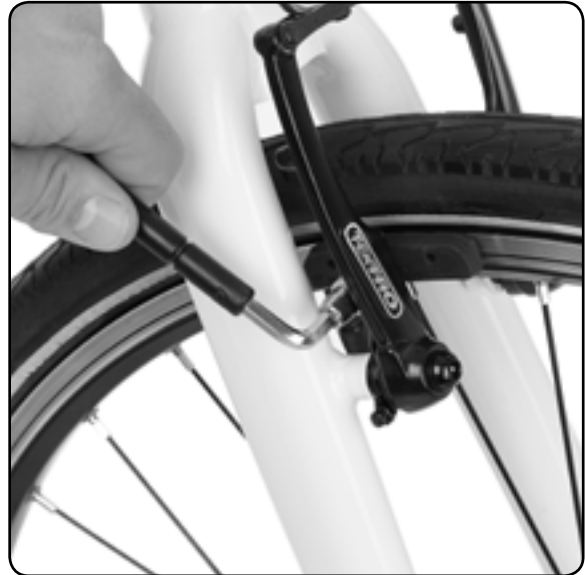
Loosen the brake pad fixing bolts.
