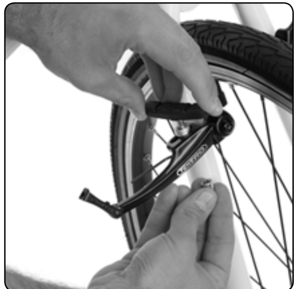
Insert the new brake pad. Screw the new brake pad into place.
