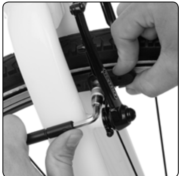
Hold the brake pad in the correct position against the wheel rim and re-tighten the screws.
