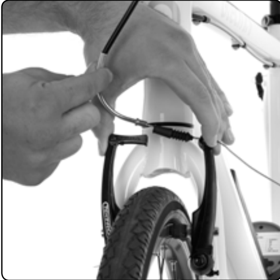
Close the brake arms using your thumb and index finger and lift out the brake cable.
