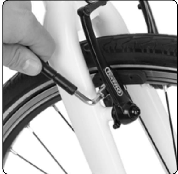
Loosen the brake pad fixing bolts.
