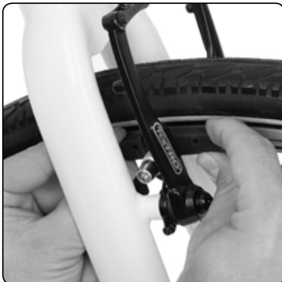
Straighten the brake pad and make sure that it is at the right height, so that the whole of its surface rests against the wheel rim when the brake arms are closed.
