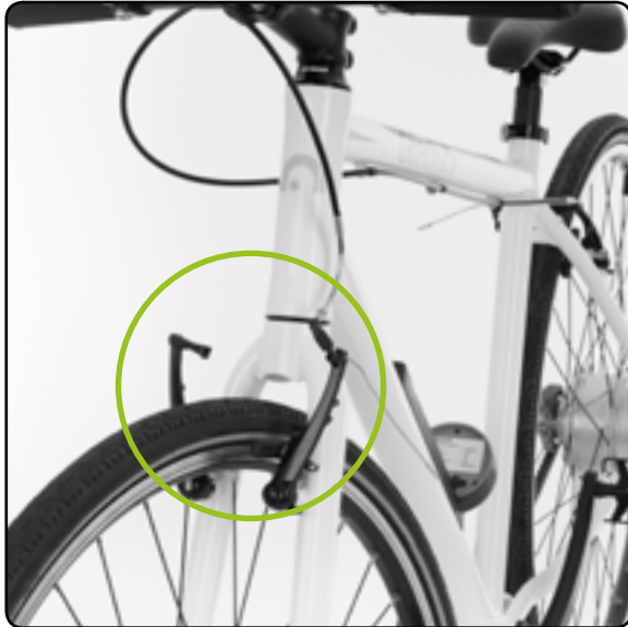
Locate the front brake arms and brake cable at the top of the front forks.
