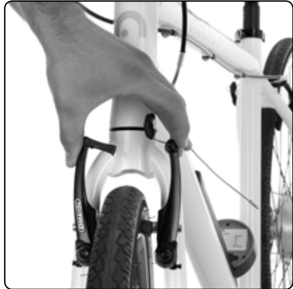
Squeeze the brake arms together
