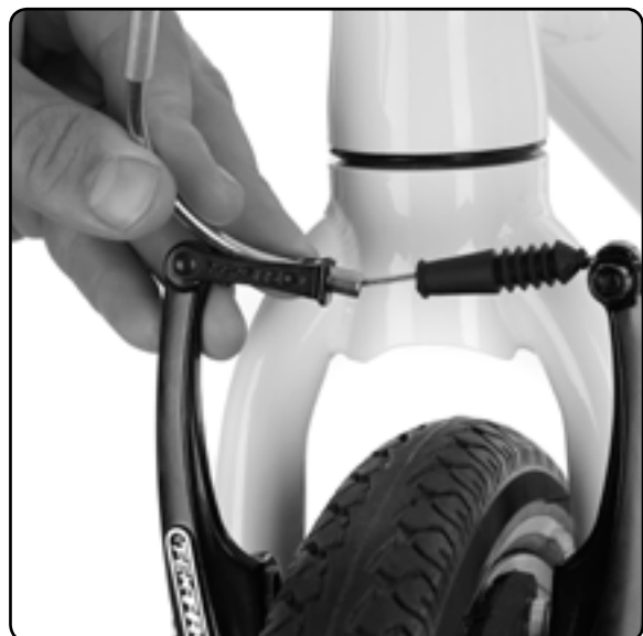
The cable should automatically pull itself into the right position, with the metal end slotting into the hole in the cable holder.
