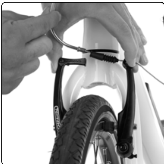
Pull the brake cable across and hook the thinner part of the cable through the gap in the cable holder. You may need to pull back the black rubber cable cover to do this. The brake cable should be tight to pull across.
