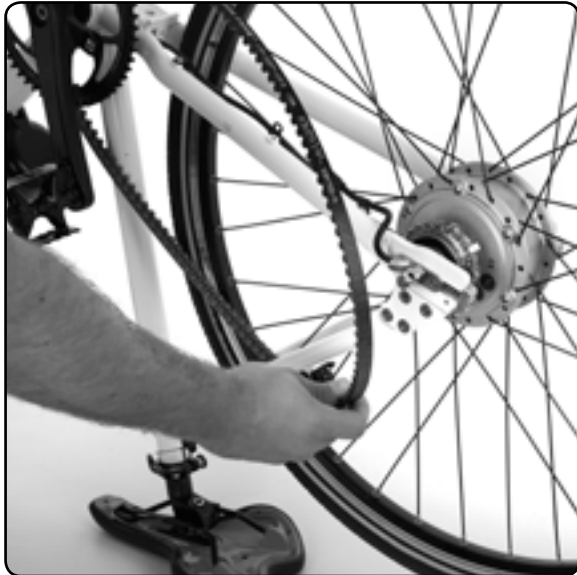
Take the drive belt off the rear wheel sprocket and move around the rear forks, away from the frame.
