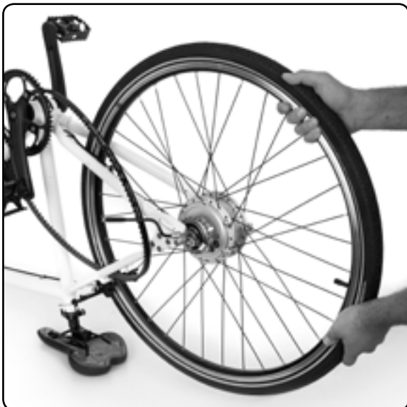
Slide the wheel backwards off the frame to remove.
