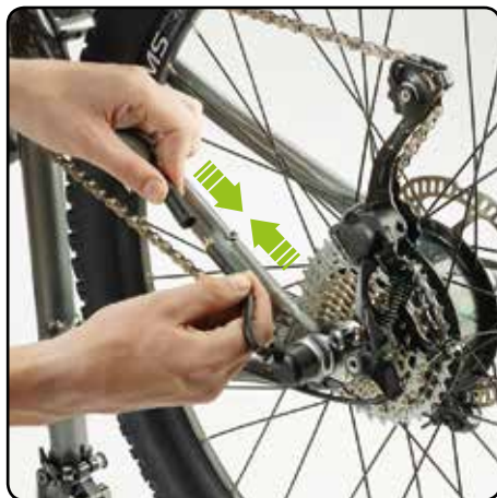
Reconnect the hub connector cable.
