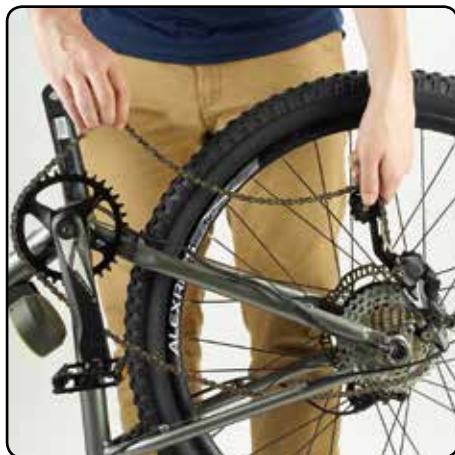
Pull the derailleur forward and feed the chain onto the front crank.
