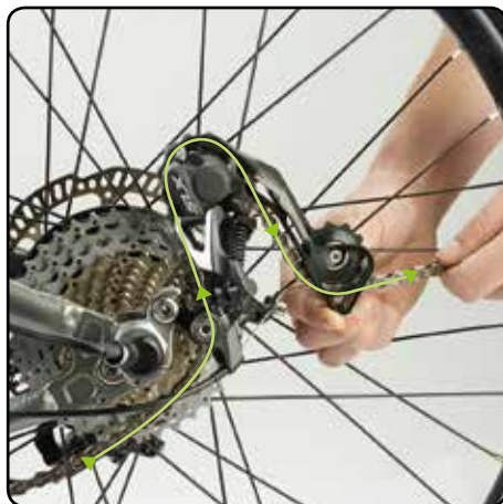
Feed the new chain through the derailleur.
