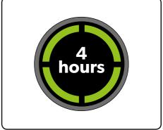
The battery can be charged from flat in 4 hours. The state-of-charge indicator will show 4 solid green lights when it is fully charged.
