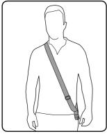
The harness is included as a safety feature for use with the branch cutter and the hedge trimmer. The sling passes over your head and rests on your shoulder - use the sliding adjuster to ensure the harness fits you comfortably.
