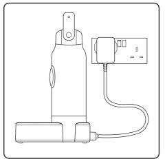
Place the battery onto the charging unit. Plug in the charger and switch it on.
