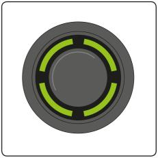
While charging, the LEDs will progressively pulse until all four are lit. When the battery is fully charged the LEDs will turn off and the charger LED will flash.
