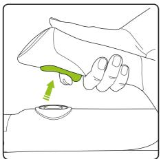
The leaf blower has variable power depending on the amount of pressure applied to the trigger. To provide more power, apply more pressure to the trigger.
