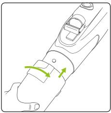
Push the nozzle over the marker and twist the nozzle clockwise over the bayonet.
