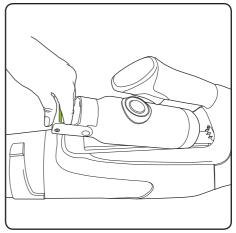
Then remove the battery from the cradle by the handle.
