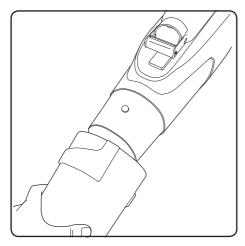
Align the bayonet on the nozzle to the marker on the main body.
