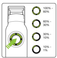
To find out how much charge there is in the battery press the button in the centre of the state-of-charge display. The number of lit LEDs shows the charge.
