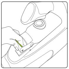
To remove the battery push the release lever in the handle to unlock the battery.
