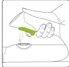
To provide less power to the leaf blower, apply lighter pressure to the trigger.
