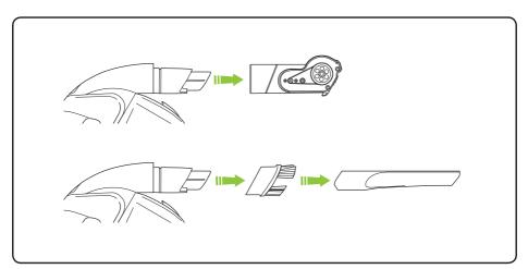
An active nozzle is built into your Multi K9. The dusting brush, crevice tool, and power brush all attach to the active nozzle.
