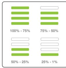
The battery state of charge indicator shows how much charge the Multi K9 has. As you use the product, the green lights will turn off in a downwards direction.
