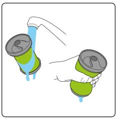
Wash the filter under a tap, squeeze it out then let it **dry completely** before using it. Use your spare filter while it dries. (You can get more at **www.gtech.co.uk**) **Never operate the Multi K9 without the filter inside the bin. You could damage the motor.**
