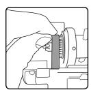
Slide the belt off the end of the brush bar drive gear.
