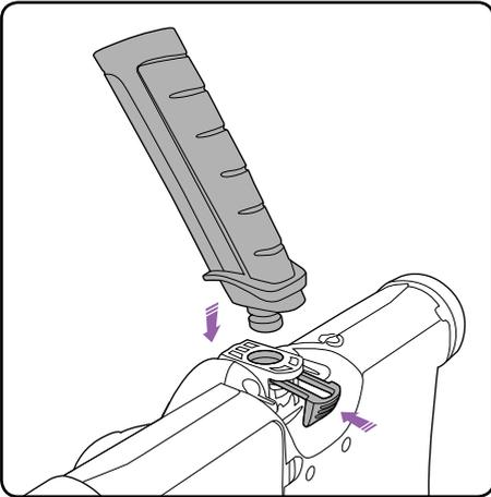
Place the lower handle into the socket.
