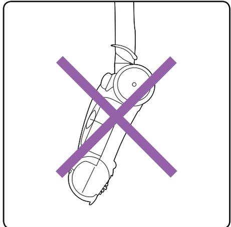
Try to avoid carrying the sweeper 'nose down' as you risk spilling dirt from the dust tray.
