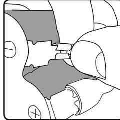
Push the latch on the connector and pull it away from the battery. Repeat for red connector.
