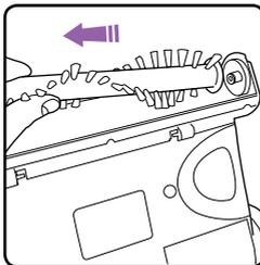
Lift the end of the brush bar, then slide out of the unit. Remove any hair, fibre and dust from the edge wheel and brush bar.
