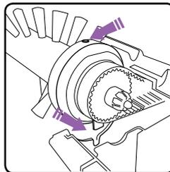
Replace the Brush Bar by fitting the shaft into the bearing in the housing, then engage the end with the drive gear into the unit. Replace belt when re-assembling.
