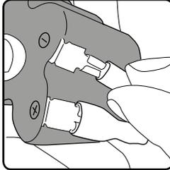
Remove the battery and locate the connectors. Starting with the black terminal, slide back the plastic cover.
