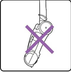
To avoid spilling dirt from the dust tray do not carry the product 'nose down'.
