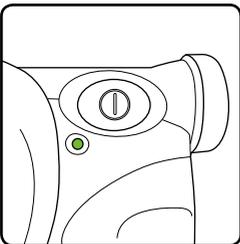
The LED indicator shows the charge level of the battery when discharging during use.
