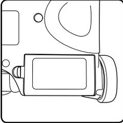
Switch off the sweeper, remove charger and dust tray and turn the sweeper over. Unclip the battery compartment.
