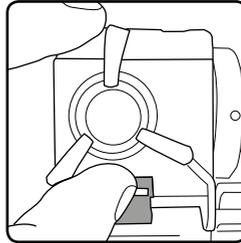
To remove the edge wheel, push the latch and pull the unit away from the body of the sweeper.
