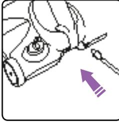
Connect the charge adaptor to the charging jack on the rear of the main unit.
