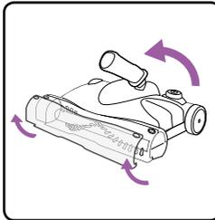
Remove the visor by simultaneously unclipping the bottom outer edges then lifting off. Push lower handle fully forward.
