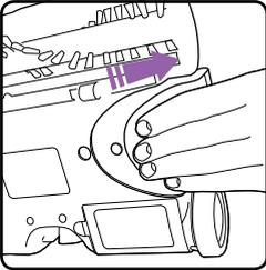
To achieve the best performance, empty the dust tray after each use. Press underneath the tray to release catch.
