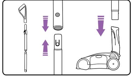
Assemble the three parts of the telescopic tube as shown, ensuring each piece clicks into place. Insert telescopic handle into lower handle until it clicks into place.
