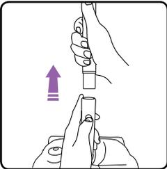
Remove telescopic handle from the lower handle by depressing button on handle and removing tube.
