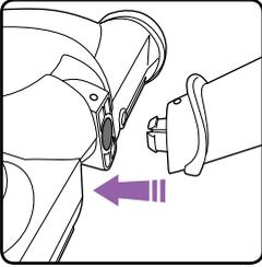
Align the dots and insert lower handle into main unit until it clicks into place.
