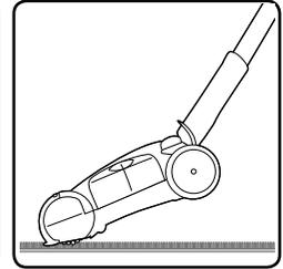
For deeper cleaning and carpet grooming, lift the handle to lower the brush bar into the carpet.
