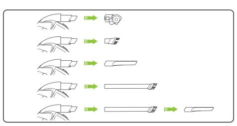
An active nozzle is built into your Multi K9. The dusting brush, crevice tool, extension tube and power brush all attach to the active nozzle.
