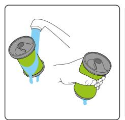
Wash the filter under a tap, squeeze it out then let it **dry completely** before using it.
