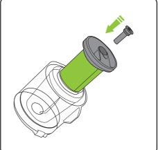
Ensure cartridge is refitted on to filter before using.
