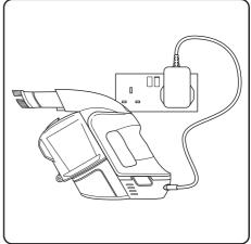
The battery can be charged on or off the main unit
