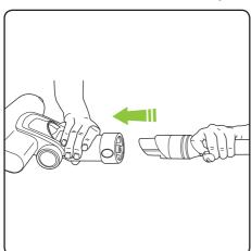
The power must be off while changing tools. Take the Power Floor head and attach it to the extension tube. The battery must be removed when changing attachments.
