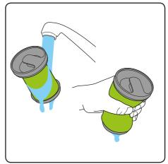
Wash the filter under a tap, squeeze it out then let it **dry completely** before using it. Recommended water temperature 40°C. Do not use any detergent or soaps. (You can buy more at www.gtech.co.uk)
