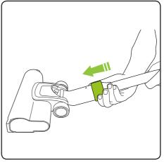
Before you remove the brush bar, you will need to remove the Power Floor head from the extension tube. Gently pull on the green locking ring attached to the Power Head to remove.
