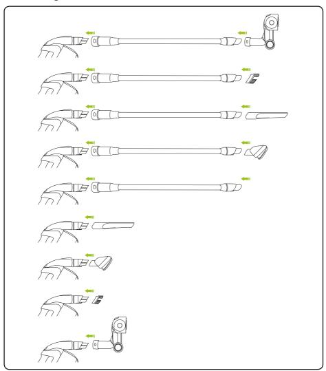
There are many configurations for the Power Floor. Refer to this diagram to see how each tool can be attached and used.
