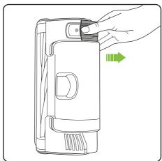
Press the latch on the top of the battery and slide it out of the battery-housing.
