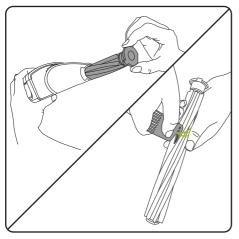
Assess the blockage. If necessary, remove the brush-bar, running the blade of the hair removal tool between the brushes to cut the strands (see p.12-13 for more information).
