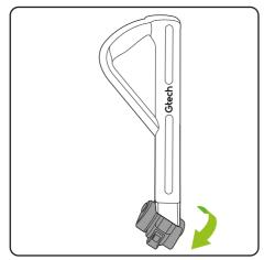
Hold the handle so that it is facing to the left and rotate the steering module so that the wheels are on the right hand side.
