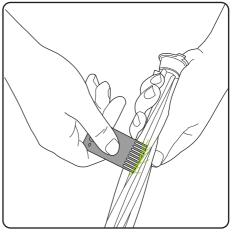
You can then use the comb end of the hair removal tool to pull the hair from the brush-bar. Never operate the HyLite without the brushbar in place.
