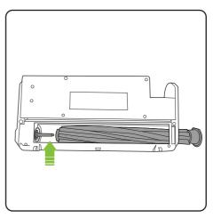
When replacing the brush-bar, ensure that it locates onto the steel pin at the other end of the head, then turn the latch to the 'locked' position.
