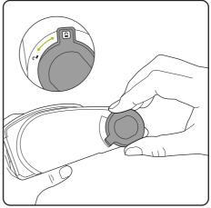
After clearing the jam, slide the brush-bar back into place and turn the latch to the 'locked' position. Ensure the brush-bar button is pushed back in. The vacuum is now ready to use again.
