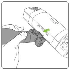
Holding the unit from the right-hand side, line the steering module up with the locking tabs on the main unit. You can't do this while the main unit is on the floor.
