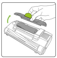
Lift and remove the bag-chamber lid.
