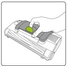
Remove the battery before removing the bag. Open the bag-chamber by lifting the latch on top of the lid.
