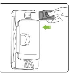
To refit the battery, line it up and slide it into the battery-housing. The battery will click into place when correctly fitted.
