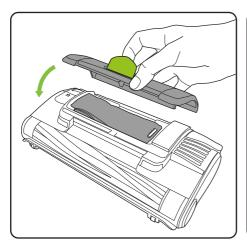
Place the lid back onto the chamber and press down. It will click into place once it is secure.
