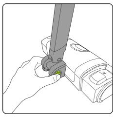
To detach the handle, squeeze the two green buttons on each side of the steering module. The handle will now unlock and can be removed from the main unit.
