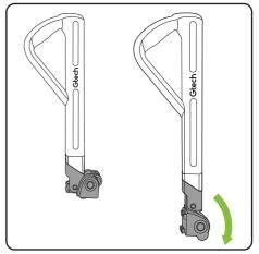
Pull the wheels down in a clockwise motion until the steering module clicks into place. The handle should now look like the image on the right.
