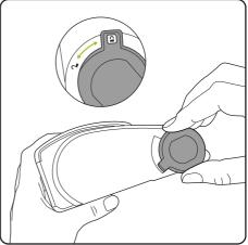
Remove the battery before maintaining any part of your HyLite. Rotate the latch from the 'locked' position to the 'unlocked' position. ۲
