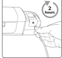
Plug the charger into the mains and connect it to the battery. Switch the power on at the mains.
