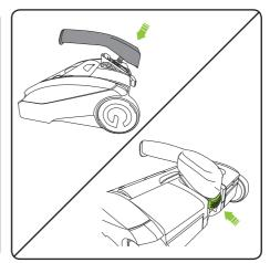
To attach the speed clean handle, insert the pin into the yoke (hole) on the AirRam head. Push the locking clip back into the head to secure the handle.
