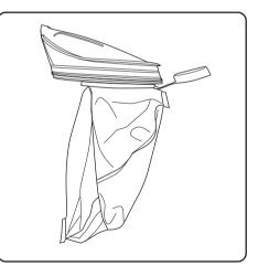
To get maximum efficiency from the bag, it is important to expand the bag before insertion. **Do not use the vacuum without a bag: it may damage the motor and will invalidate your warranty.**
