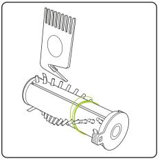
To remove hair from the brush bar, run the hair removal tool down the groove to cut the hair, then pull it out. Never operate the power head without the brush bar in.
