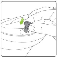
Slide the scented cartridge into the opening on the right side of the lid.
