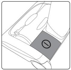
The power button is located on the left hand side of the AirRAM head assembly.
