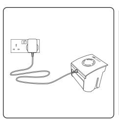
Plug the charger into the mains and connect it to the battery. Switch on at the mains.
