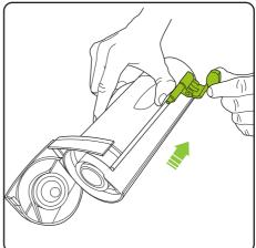
Pull the green lever back towards the bottom of the bin. Close the bin lid and reinsert the bin into the AirRAM.
