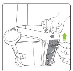
Re-insert the brush bar, starting by the end furthest away from the button. Then line up and push the brush bar into the AirRAM until it clicks into place.
