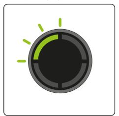
When the state of charge indicator starts to flash one green LED, recharge the battery.
