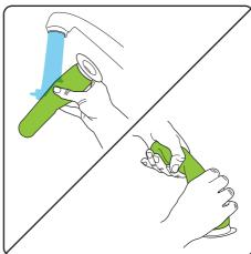
Wash the filter under a tap. Squeeze out any excess water then let it **dry completely** before reinserting into the AirRAM. Recommended water temperature 40°C. Do not use detergent or soaps. **Never put bin back without filter inside. You could damage the motor.**
