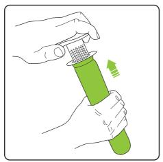
Slide the filter onto the inner shroud.
