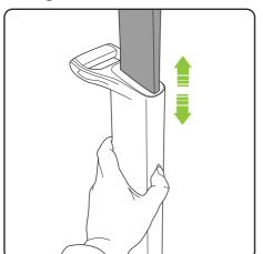
To stow or extend the upper handle simply press the button on the lower handle to unlock the upper handle.
