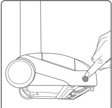
Rest the AirRAM on its side and locate the brush bar button on the right hand side. Press the button inwards and then pull the brush bar out from the bottom of the AirRAM.
