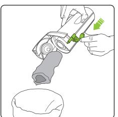
Hold the AirRAM's bin over a rubbish bin and push the green lever towards the lid to empty the dirt.
