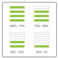
The battery state of charge indicator shows how much charge the Multi K9 has. As you use the product, the green lights will turn off in a downwards direction.
