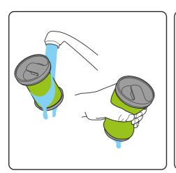
Wash the filter under a tap, squeeze it out then let it **dry completely** before using it. Recommended water temperature 40°C. Do not use detergent or soaps. Use your spare filter while it dries.
