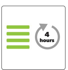
After 4 hours, the LEDs turn solid green and charging is complete.
