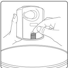
Hold the Multi K9's bin over a rubbish bin and release the latch to empty the dirt. A gentle tap will help. Remove the filter and tap off the excess debris each time you empty the bin.
