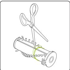
To remove hair from the brush bar, run an open pair of scissors down the groove to cut the hair, then pull it out. Never operate the power brush without the brush bar in.
