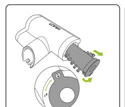
To clean the brush bar, first remove the power brush. Rotate the latch from the lock to the unlock position and pull out the brush bar.
