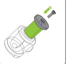
Ensure tab is refitted on to filter before using.
