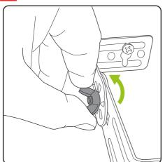
To adjust the angle of the heater, loosen the wing nuts.
