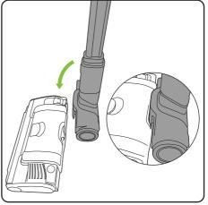
To attach the handle to the main unit there is no need to lift the vacuum from the floor. Just push the hook on the steering module into the latch at the back.
