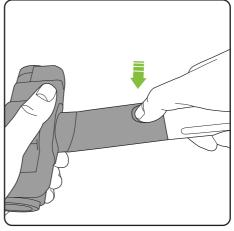
To remove the steering module press the button and pull the handle out.
