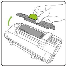
Lift and remove the bag-chamber lid.
