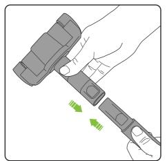
To fit the steering module to the handle simply push the end of the handle into the neck of the steering module until it clicks into place.
