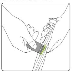
You can then use the comb end of the hair removal tool to pull the hair from the brush-bar. Never operate the product without the brushbar in place.
