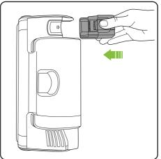
To refit the battery, line it up and slide it into the battery housing. The battery will click into place when correctly fitted.
