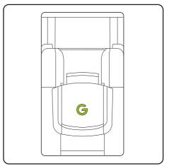
Whilst charging, the 'G' on the battery will pulsate green. When fully charged, it will show a solid green colour.
