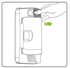
Press the latch on the top of the battery and slide it out of the battery-housing.
