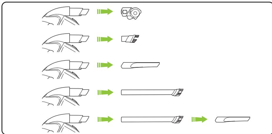
An active nozzle is built into your Multi. The dusting brush, crevice tool, extension tube and power brush all attach to the active nozzle.
