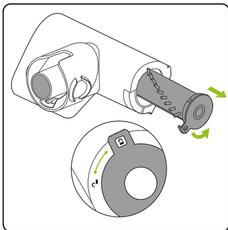
To clean the brush bar, first remove the power brush. Rotate the latch from the lock to the unlock position and pull out the brush bar.
