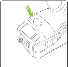
The LED light (7) will illuminate when the trigger is depressed. It will automatically shut off the light when the tool is not in use. The light will stay on for a few seconds after the
