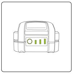
The state of charge of the battery can be tested by pressing the button. Three bars indicates a full charge, two bars a partial charge, one bar low charge.
