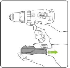
To install, simply insert the battery pack.
