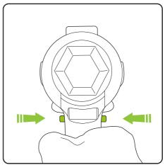
Set the forward/reverse switch (9) in the OFF (Centre lock) position to lock the trigger and help prevent accidental starting when not in
