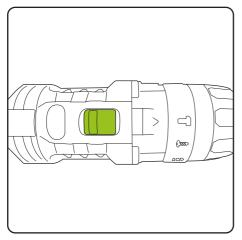
The speed of the drill can be changed for various applications. Press the speed selector (1) button to change to the desired speed.
