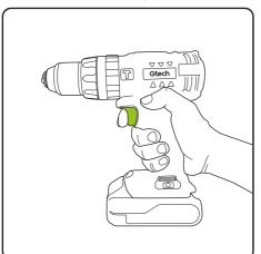
The variable speed trigger (6) delivers higher speed with increased trigger pressure and lower speed with decreased trigger pressure. To turn on the tool, depress the trigger. To turn it off, release the trigger and allow the tool to come to a complete stop.
