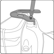
To install, insert the clip into the groove in the housing and fasten it with screw.
