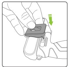
The belt clip (8) may be installed on either side of the tool.
