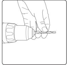
To remove the bit, turn the chuck sleeve clockwise to release.
