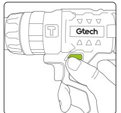
Push the forward/reverse switch (9) to the left of the trigger for forward operation. Push the switch to the right to reverse the direction. The tool will not run unless the direction of rotation switch is pushed fully to the left or right. product is switched off.
