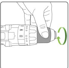
Turn the chuck sleeve (4) counterclockwise (as viewed from the front) to open the chuck jaws. Place the driver/drill bit into the chuck as far as it goes. Turn the sleeve clockwise to tighten the chuck.
