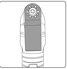
Never attach the blade with the cutting edge pointing backwards.
