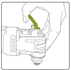
Flip up the tool clamp lever at the head of the product, and push the lever forwards.
