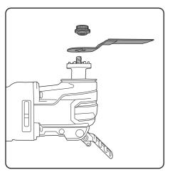
Place the desired tool into the tool holder paying attention to the direction in which the tool is pointing then replace the locking nut at finger-tightness.
