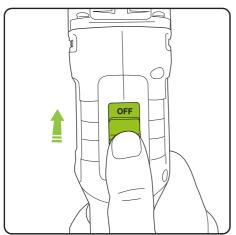
The on/off switch is a sliding button. The product will remain on when it has been pushed into the on position.
