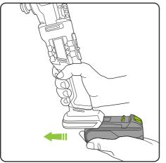
To install, simply insert the battery pack.
