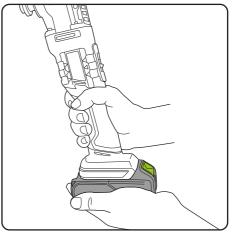
Make sure the latch on the battery snaps in place and battery pack is secured to the tool.
