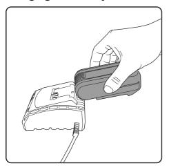
To charge the battery, line up the slot of the battery with the slot of the charger and slide into place. **Charger is sold separately.**
