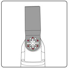
Ensure the pins on the tool holder align correctly with the holes in the tool.
