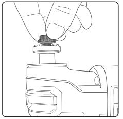
While the tool clamp is in the released position you can undo the locking nut with your fingers
