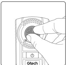
There is an adjuster on the lens to turn the beam from wide to narrow.
