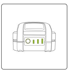
The state of charge of the battery can be tested by pressing the button. Three bars indicates a full charge, two bars a partial charge, one bar low charge.
