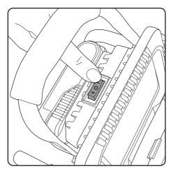
The power switch is on the top of the light. There are two intensity settings.
