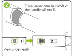
When the pole is fully inserted, the button (1) will pop up into the aperture (2)
