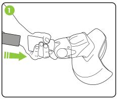
Insert the body pole into the grass trimmer head, ensuring it is the right way up.
