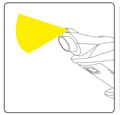
There is a LED headlight on top of the product to illuminate the area being cleaned.
