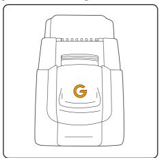
If the brush bar has jammed or there is a blockage, the battery will display a solid amber light for 5 seconds.
