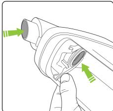
Remove the battery and bag and look through the nozzle. Remove any blockages.
