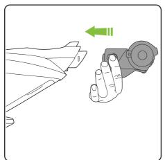
To attach the power brush, slot it over the standard nozzle. The power must be off while changing nozzles. To remove, place your fingers in the indents of the attachment, grip and pull it away from the main unit.
