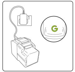
Whilst charging, the 'G' on the battery will pulsate green. Once the battery is fully charged, the indicator will show a solid green colour. This will take up to 2 hours from flat.
