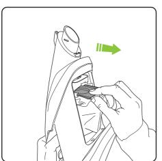
Slide the bag out of the bag chamber by gripping the collar of the bag.
