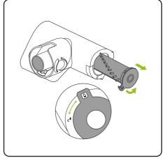
To clean the brush bar, first remove the power brush. Rotate the latch from the 'locked' to the 'unlocked' position and pull out the brush bar.
