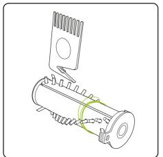
To remove hair from the brush bar, run the hair removal tool down the groove to cut the hair, then pull it out. Never operate the power head without the brush bar in.
