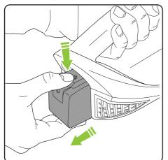
Press the latch on top of the battery downwards and slide it out of the product.
