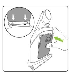
Refit the chamber cover. Fit the pegs on the cover into the slots at the bottom, then push the top part of the cover. You will hear a click when the cover is correctly fitted.
