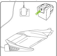
Connect the charger to the charging port located on the back of the battery pack. Plug the charger into the mains socket. You can charge the battery both on and off the product.
