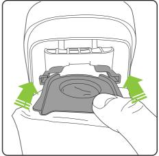
Slide the bag collar into the grooves inside the bag chamber. Make sure the collar is completely inserted into the chamber and the bag has expanded. A reduction in suction will occur if the bag has not expanded or is incorrectly fitted.
