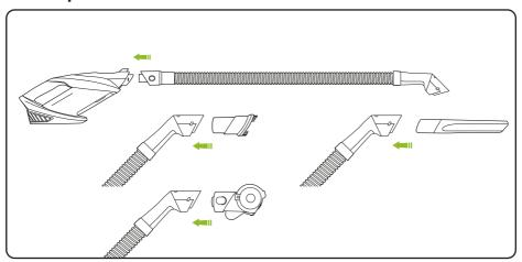
The flexible power hose attaches in the same way as the other accessories and can be used as it is or with the addition of other tools.
