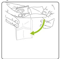
Before placing the bag in the chamber, ensure the bag is fully expanded by gently unfolding and spreading the fabric of the bag.
