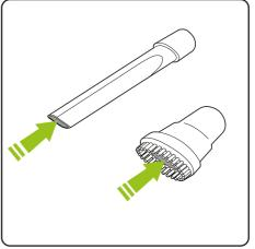
The tools can block sometimes too, so remove these from the main unit before checking for blockages.
