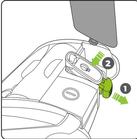
Pull out the green locking clip to allow the lower handle to fit (the clip remains attached to the head) Insert the metal pin on the lower handle into the hole in the pivot yoke.
