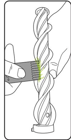
To remove hair from the brush bar, run the hair removal tool down the groove to cut the hair, then use the comb remove it. Never operate the product without the brush bar in place.
