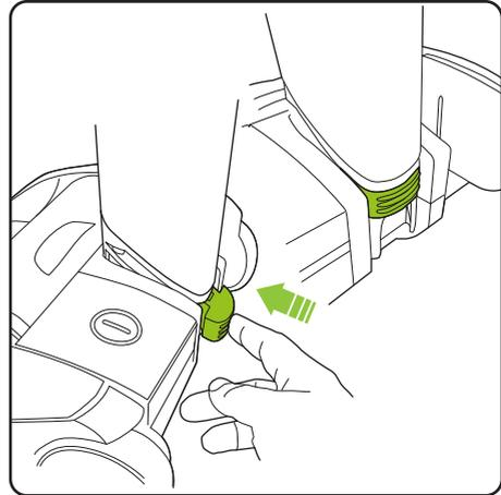
Ensure the lower handle is sitting completely flush against the pivot yoke. Firmly push the green locking clip until it clicks fully into place. The clip can be pulled out to unlock the lower handle should it need to be removed.
