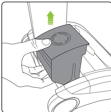
To remove the battery, squeeze the latch underneath and pull upwards.
