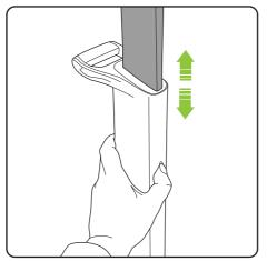
To stow or extend the upper handle simply press the button on the lower handle to unlock the upper handle.
