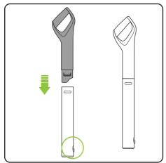
Push the two parts of the upper handle together in the orientation shown above. They will only fit one way. They will click into place and remain permanently fixed.
