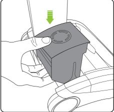
It is OK to charge for 1 hour for a burst of cleaning. Replace the battery by sliding it down into the head assembly. It will click into place.
