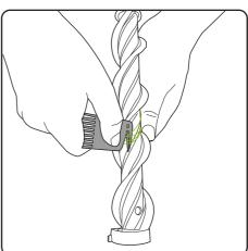
To remove hair from the brush bar, run the hair removal tool down the groove to cut the hair.
