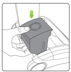
Replace the battery by sliding it down **into the** head assembly.
