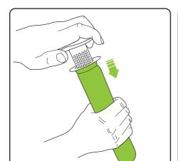
Remove the filter from the inner shroud, by twisting and pulling.
