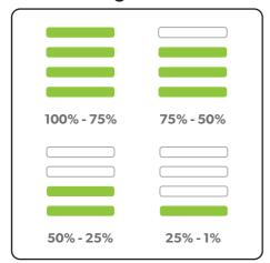
The battery state of charge indicator shows how much charge the battery has. As you use the product, the green lights will turn off in a downwards direction.
