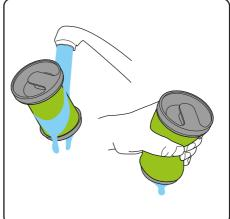
Wash the filter under a tap, squeeze it out then let it **dry completely** before using it. Recommended water temperature 40°C. Do not use detergent or soaps. (You can buy more at **www.gtech.co.uk**)
