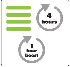
After 4 hours, the LEDs turn solid green and charging is complete. It is OK to charge for 1 hour for a burst of cleaning.
