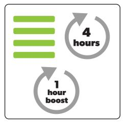
After 4 hours, the LEDs turn solid green and charging is complete. It is OK to charge for 1 hour for a burst of cleaning.
