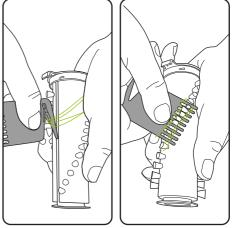
To remove hair from the brush bar, run the hair removal tool down the groove to cut the hair, then pull it out with the comb. Never operate the power head without the brush bar in.
