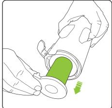
Pull the filter out of the filter housing. Tap the dirt from the filter and tip any dirt from the filter housing. Wash the filter if necessary.
