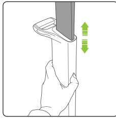
To stow or extend the upper handle simply press the button on the lower handle to unlock the upper handle.
