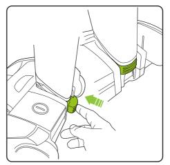
Ensure the lower handle is sitting completely flush against the pivot yoke. Firmly push the green locking clip until it clicks fully into place. The clip can be pulled out to unlock the lower handle should it need to be removed.
