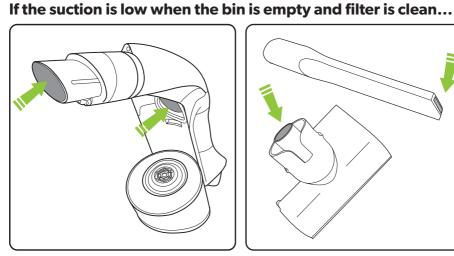
...you have a blockage. Remove the battery & bin and look through both ends of the tube. Remove any blockages.
