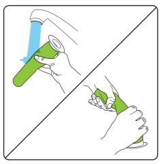
Wash the filter under a tap. Squeeze out any excess water then let it dry completely before reinserting into the product. Recommended water temperature 40°C. Do not use detergent or soaps. Never put the bin back without filter inside. You could damage the motor.
