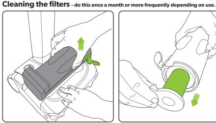
Holding onto the head with one hand, pull the bin handle and lift the bin out of the product.
