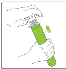
Slide the filter onto the inner shroud.
