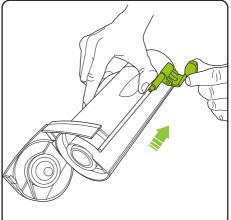
Pull the green lever back towards the bottom of the bin. Close the bin lid and reinsert the bin into the product.
