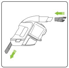
The dusting brush can be slotted onto the active nozzle. The crevice tool is stored on board the product for easy access.
