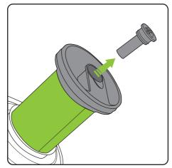
Remove the old scented cartridge by pulling it out from the housing at the top of the filter.
