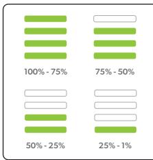
The battery state of charge indicator shows how much charge the product has. As you use the product, the green lights will turn off in a downwards direction.
