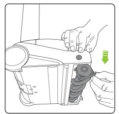
The brush bar can now be removed, starting at the button end.
