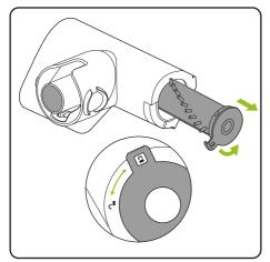
To clean the brush bar, first remove the power brush. Rotate the latch from the lock to the unlock position and pull out the brush bar.
