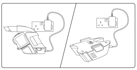
The battery can be charged on or off the main unit
