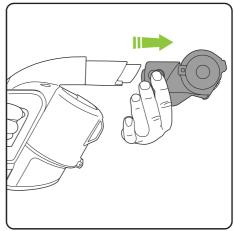
Gently pull the Power Brush from the product to remove. The battery should be removed when changing attachments.
