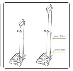
The upper handle can be set in two positions: Lowered for storage and raised for use. To lower the handle, release the upper button. To raise the handle from the stored position, release the lower button.
