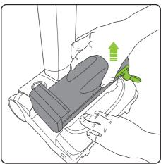
Holding onto the head with one hand, pull the bin handle and lift the bin out of the product.
