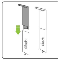
Push the two parts of the lower handle together in the orientation shown above. They will only fit one way. They will click into place and remain permanently fixed.
