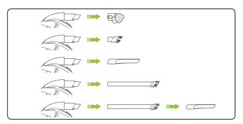
An active nozzle is built into your product. The dusting brush, crevice tool, extension tube and power brush all attach to the active nozzle.
