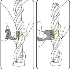
To remove hair from the brush bar, run the hair removal tool down the groove to cut the hair, then use the comb remove it.
