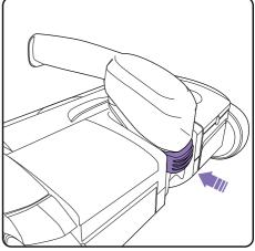
Push the purple locking clip back into the head to secure the handle.
