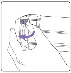
Lift and release the latch marked with the purple arrow to pull open the lid.
