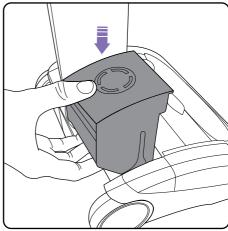
Replace the battery by sliding it down **into the head assembly.**It will click into place.
