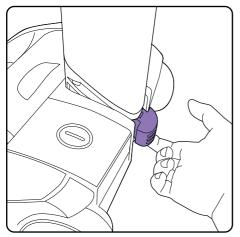
Remove the AirRAM handle by pulling out the purple locking clip (at the base of the lower handle) until you feel it come loose.
