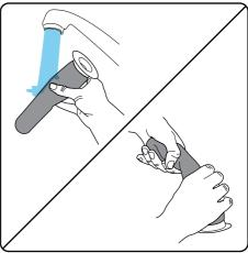
Wash the filter under a tap. Squeeze out any excess water then let it **dry completely** before reinserting into the product. Recommended water temperature 40°C. Do not use detergent or soaps. **Never put bin back without filter inside. You could damage the motor.**
