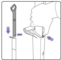
Insert the upper handle into the lower handle. You will need to press the button on the upper handle to fit it in. Once it slides down you will hear it click into place.
