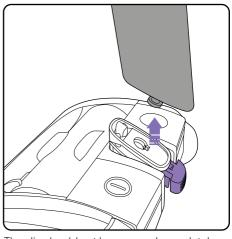
The clip should not be removed completely as it remains part of the lower body assembly.
