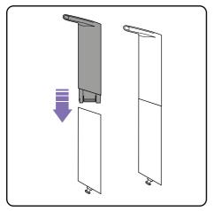
Push the two parts of the lower handle together in the orientation shown above. They will only fit one way. They will click into place and remain permanently fixed.
