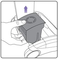
To remove the battery, squeeze the latch underneath and pull upwards.
