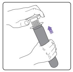
Slide the filter onto the inner shroud.
