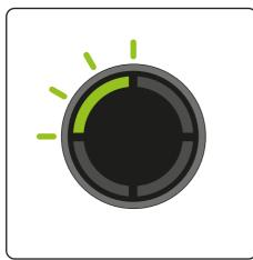
When the state of charge indicator starts to flash one green LED, recharge the battery.
