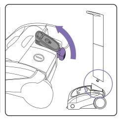
Push the pivot yoke to the upright position. This might require some force. Attach the lower handle to the head assembly
