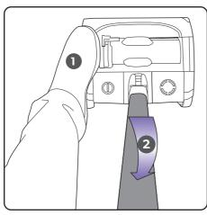
Without pressing the power button, place your foot on the left side of the head (1) and pull the handle back (2).
