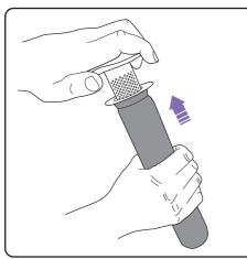
Slide the filter onto the inner shroud.
