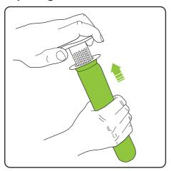
Slide the filter onto the inner shroud.
