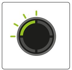
When the state of charge indicator starts to flash one green LED, recharge the battery.
