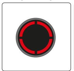
If the brush bar jams during use, the product will stop and the LEDs will appear red. You will need to remove and clean the brush bar.
