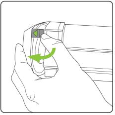
Lift and release the latch marked with the green arrow to pull open the lid.
