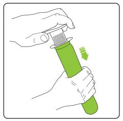
Remove the filter from the inner shroud, by twisting and pulling.
