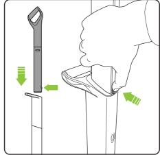
Insert the upper handle into the lower handle. You will need to press the button on the upper handle to fit it in. Once it slides down you will hear it click into place.
