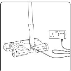
Plug in the charger and connect the jack to the socket at the rear of the sweeper. A full recharge will take 6 hours. Do not charge for longer than 24 hours.
