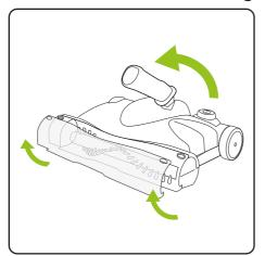
Remove the visor by unclipping the bottom outer edges at the same time then lifting off. Push lower handle fully forward.
