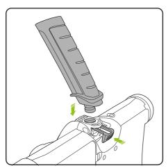
Place the lower handle into the socket. Push the locking clip back into place. Push handle forward.
