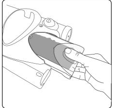
Remove the dust tray by pinching the window slightly, and pulling out.
