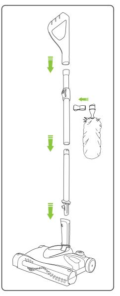
The three parts of the telescopic handle also click into place. The duster can be clipped onto the back of the handle.
