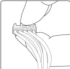
Remove the pad from the battery compartment then, pinching the clip, pull the 5-pin connector from the sweeper.
