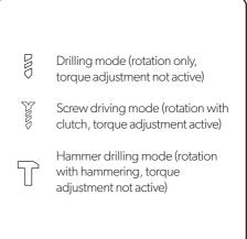
The tool is equipped with three modes for different applications. Turn the mode selector ring (2) to select the desired mode. Drill mode should be used for drilling and other heavy-duty applications. Hammer mode should be used for hammer drilling. Drive mode should be used for driving screws.
