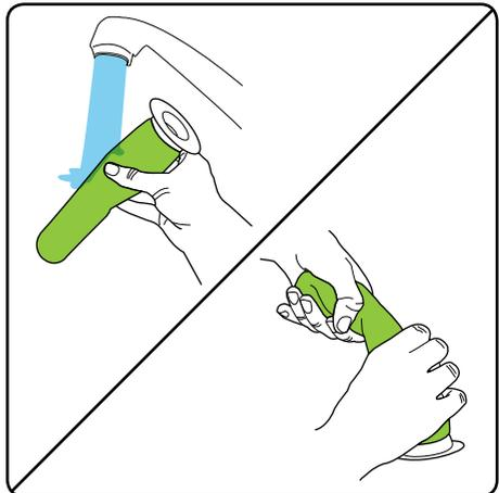
Wash the filter under a tap. Squeeze out any excess water then let it **dry completely** before reinserting into the AirRam.
