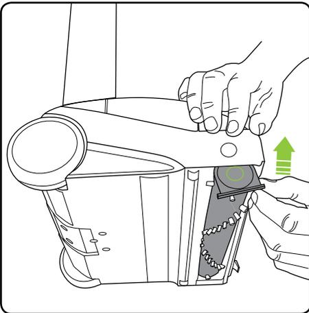
Re-insert the brush bar, starting by locating the end furthest away from the button. Then push the brush bar into the AirRam until it clicks into place.
