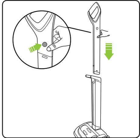
Press the button at the top of the upper handle and slot it into the lower handle until it clicks.
