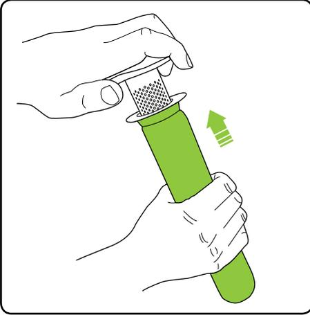
Slide the filter onto the inner shroud.
