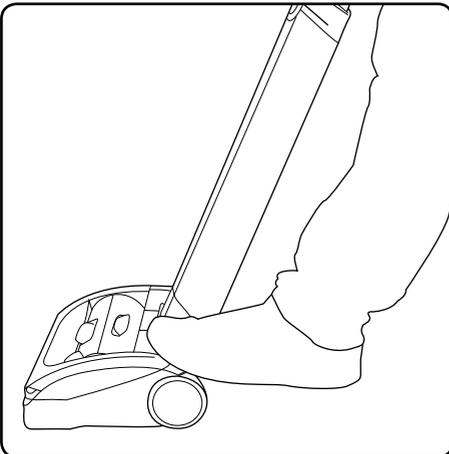
Press the button with your foot to turn the AirRam on.
