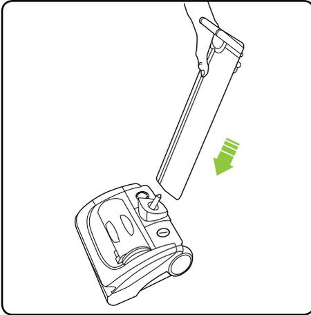
Attach the lower handle onto the head of the AirRam.
