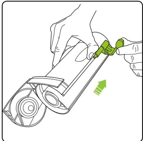
Pull the green lever back towards the bottom of the bin. Close the bin lid and reinsert the bin into the AirRam.
