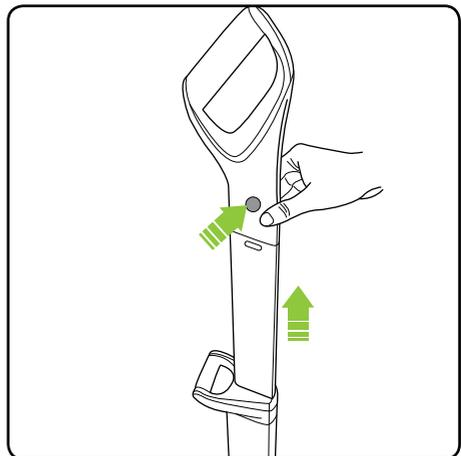
To extend the upper handle, hold down the button on the left hand side and pull it up. It will click into place.
