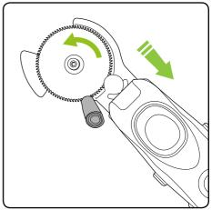
When cutting with a pulling motion the branch will rest on body of the cutter head.
