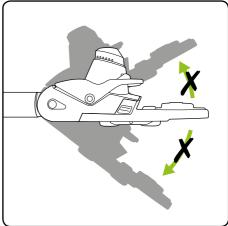
The branch cutter is not intended to pivot and must be used straight.
