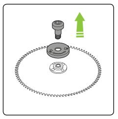
Remove the screw and the hub.
