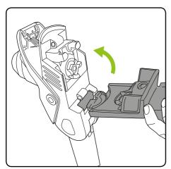
Connect branch cutter to head. It will snap into place just like the hedge trimmer blade.
