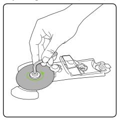
Replace the bolt and hub, tighten by turning **anticlockwise**.
