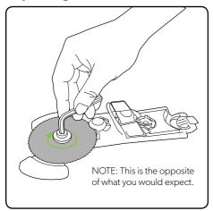
Remove the attachment from the product. Using 6mm allen key, unscrew the bolt in the hub in a **clockwise** direction.
