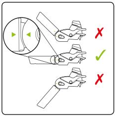
The blade will not attach unless the body is in line with the head and the arrows align.
