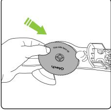
Lift the old blade out taking care of the teeth on Put new blade in. The upper face of the blade is marked clearly on the blade.
