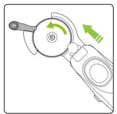
When cutting branches with front, branch will rest on support as indicated.
