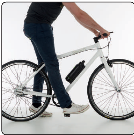
Try to reach the pedal with your heel when it is in the bottom position. Your knee should be more or less fully straight.
