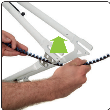
Feed the new belt through the gap in the dropout.
