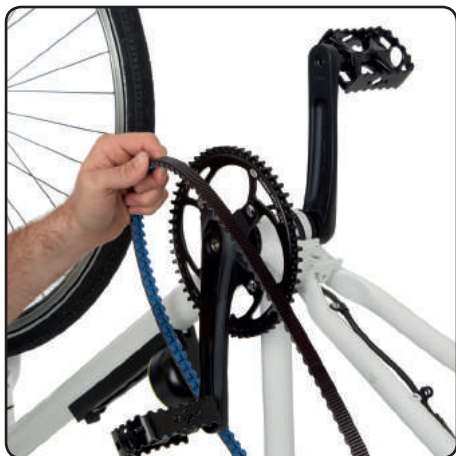
Take the belt off the pedal sprocket.
