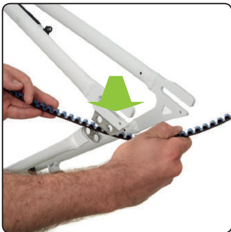
Feed the belt through the gap towards you to remove the belt.
