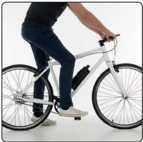
Place the balls of your feet on the centre of the pedal. If your knee is now slightly bent, the saddle height is correct.
