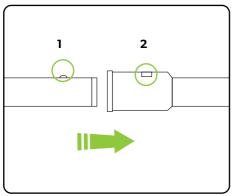
Assemble the two parts of the handle. When the pole is fully inserted, the button (1) will pop up into the aperture (2).
