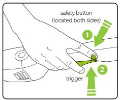
Release the button and ensure the handle clicks Push and hold the safety button on either side, then press the trigger to operate. When you release the trigger the trimmer will stop.
