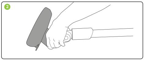
The head only rotates in one direction.
