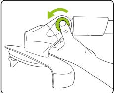
Push the green button and rotate the head to the required angle.
