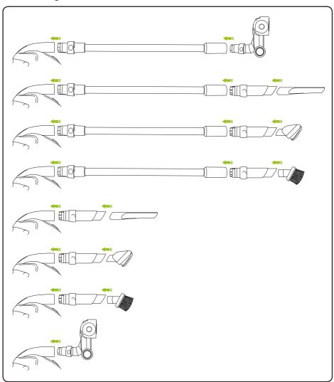
There are many configurations for the Power Floor, most of which involve the nozzle. Refer to this diagram to see how each tool can be used.
