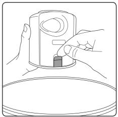
Hold the Power Floor bin over your rubbish bin and release the latch to empty the dirt.
