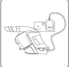
Plug the charger in and connect it to the battery.
