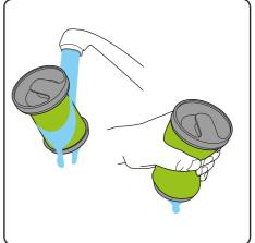
Wash the filter under a tap, squeeze it out then let it dry completely before using it. (You can get more at www.gtech.co.uk)
