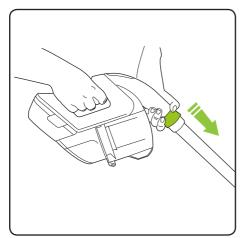
Remove the extension tube from the Power Floor by pulling gently on the green locking ring.
