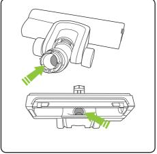
The powered floor head can also get blocked. To check for blockages thoroughly, remove the brush bar. (See page 8)
