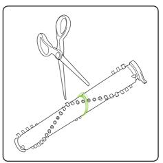
To remove hair from the brush bar, run an open pair of scissors down the groove to cut the hair, then pull it out.
