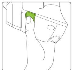
Press the green buttons and pull to remove the battery. The battery can be charged on or off the main unit. If you want to buy a spare battery go to www.gtech.co.uk or call 01905 345 891
