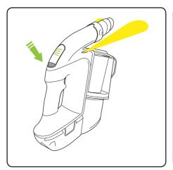
Push the button to switch the Power Floor on. Push again to switch off.
