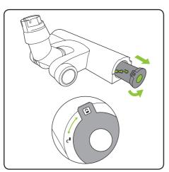
Rotate the latch on the side of the powered floor head and pull out the brush bar.
