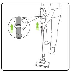
Attach the extension tube to the Power Floor K9, making sure the white dots are aligned. It will click into place.
