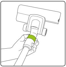
Before you remove the brush bar, you will need to remove the power floor head from the extension tube. To do this, gently pull on the green locking ring.
