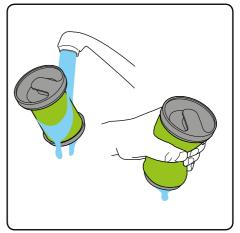
Wash the filter under a tap, squeeze it out then let it **dry completely** before using it. (You can get more at **www.gtech.co.uk**) **Never put the bin back without the filter inside. You could damage the motor.**
