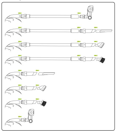
There are many configurations for the Power Floor K9, most of which involve the nozzle. Refer to this diagram to see how each tool can be used.
