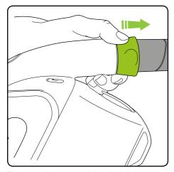
To attach the powered floor head, remove the nozzle by pulling gently on the green locking ring until the nozzle comes free from the body. The power must be off while changing tools.
