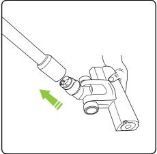
Take the powered floor head and attach it to the extension tube. It will click into place.
