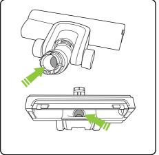
The powered floor head can also get blocked. To check for blockages thoroughly, remove the brush bar. (See page 8)
