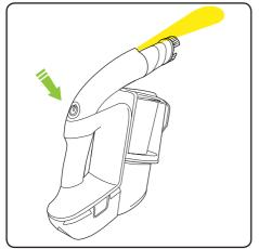
Press the button above the handle to turn the Power Floor K9 on and off.
