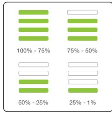
The battery state of charge indicator shows how much charge the Power Floor K9 has. As you use the product, the green lights will turn off in a downwards direction.
