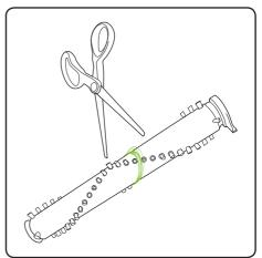
To remove hair from the brush bar, run an open pair of scissors down the groove to cut the hair, then pull it out. Never operate the Power Floor K9 head without the brush bar in.
