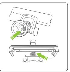
The Power Floor K9 head can also get blocked. To check for blockages thoroughly, remove the brush bar. (See page 9)
