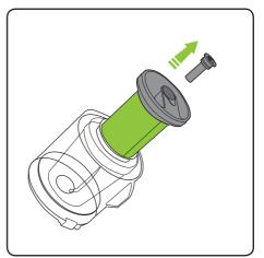
Before washing the filter, you will need to remove the scented cartridge by pulling it out from the scented cartridge housing at the top of the filter.
