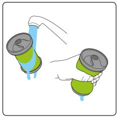
Wash the filter under a tap, squeeze it out then let it **dry completely** before using it. Use your spare filter while it dries. (You can get more at **www.gtech.co.uk**) **Never operate the Power Floor K9** without the filter inside the bin. You could damage the motor.
