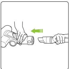
The power must be off while changing tools. Take the Power Floor K9 head and attach it to the extension tube. The battery must be removed when changing attachments.
