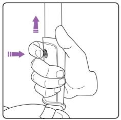
Remove the telescopic handle by pressing the button at the front of the lower handle and pulling the tube out.
