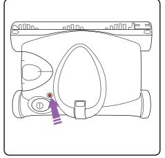
The 3 colour LED shows red when charging starts, yellow when partially charged and green when fully charged. This will only take around 3 hours.
